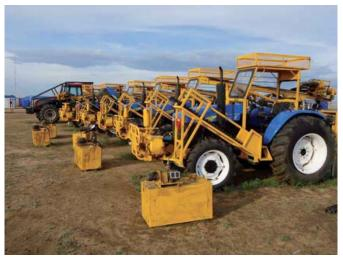
Tractor drilling rigs during seismic operations, Ethiopia.
